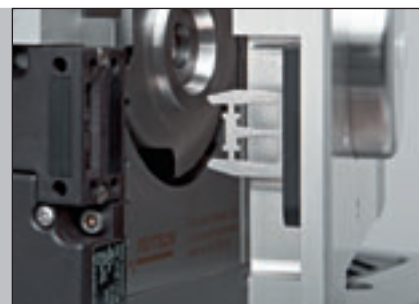
Closes particularly securely: the grinding chamber safety lock
